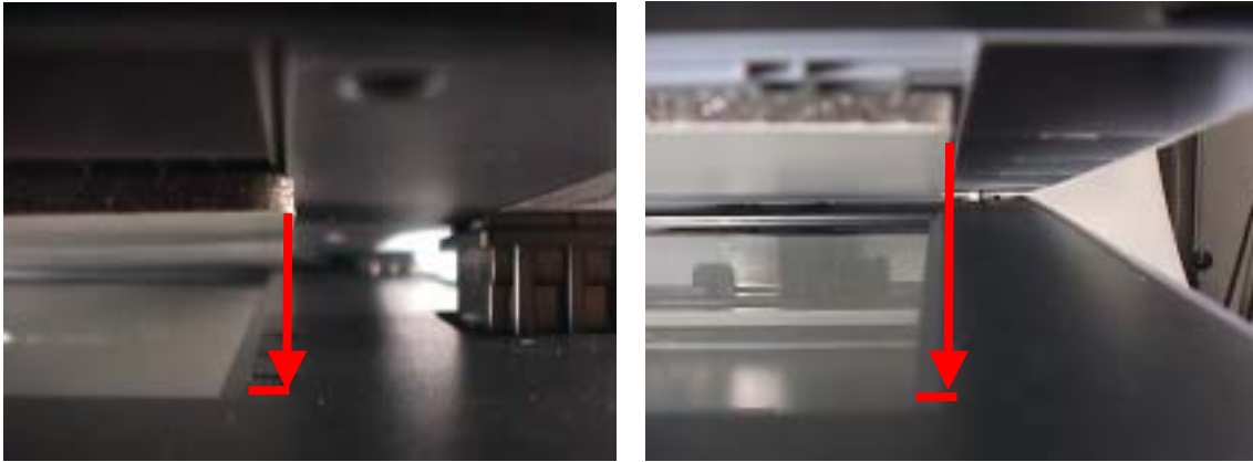
Figure1-19 Location confirmation to apply the white sheet (the rear side and the right side) (NG example)
