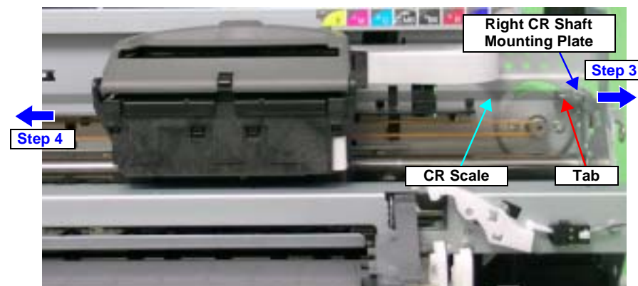
Figure 4-38. Drawing Out the CR Scale
