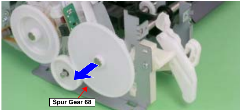
Figure 4-91. Removing the Spur Gear 68
