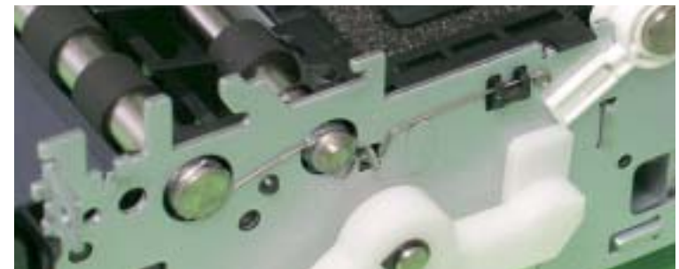
Figure 4-115. Reinstalling the EJ Grounding Spring
